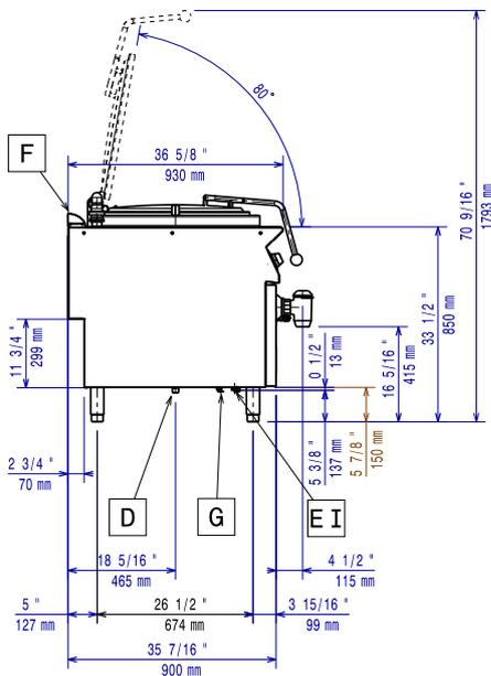
CWII = Raccordement eau froide      HWI = Raccordement eau chaude
